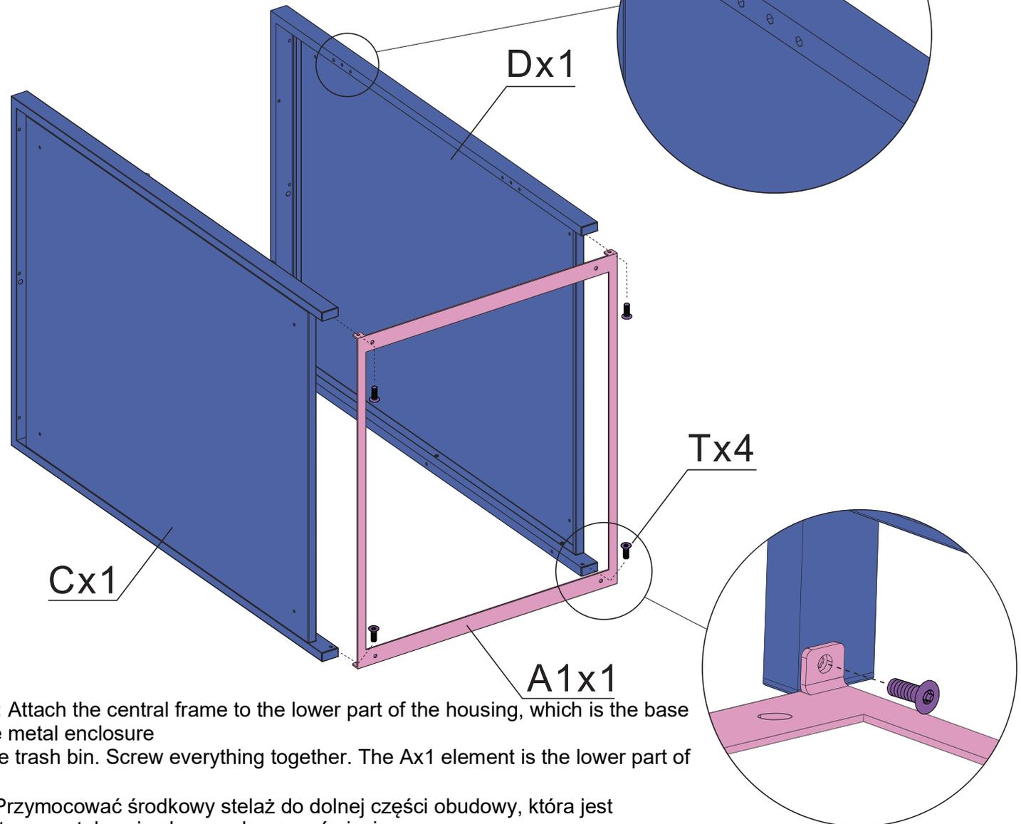
**ENG:** Attach the central frame to the lower part of the housing, which is the base of the metal enclosure for the trash bin. Screw everything together. The Ax1 element is the lower part of
