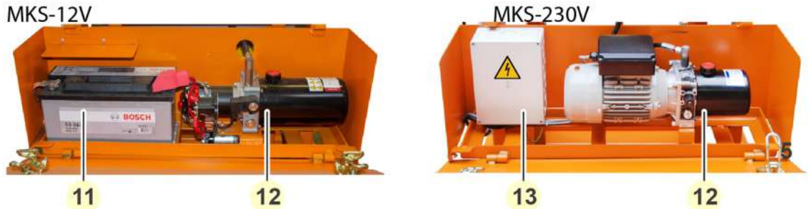
Fig. 3-3: Assemblies - box with electrohydraulic components and control panel
